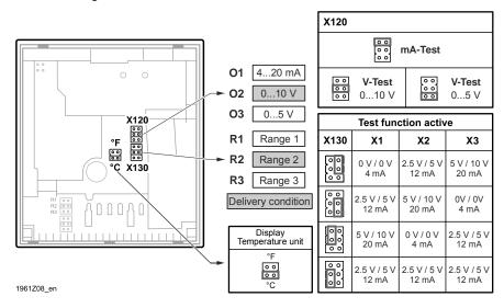
The setting elements can be accessed after removing the mounting base.
